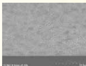
焼成後の断面SEM像 Cross-sectional SEM image after Cu film ギ酸リフロー焼成 (250°C,10min) Vacuum reflow in formic acid atmosphere
