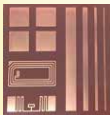
PI上の銅回路と配線形状 Cu circuit pattern on PI and line profile 膜厚 Thickness of the film : 35μm 線幅 Line width : 1mm
